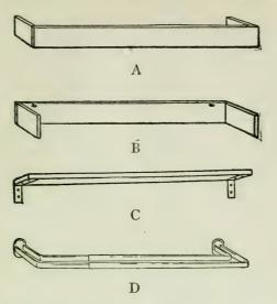
A deep valance board is shown in sketches A and B. C shows a narrow board with brackets and D is a double goose-neck rod.
